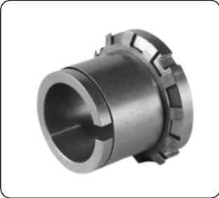
FX 90 • Low-medium torque • Short length • Self-centering • Low surface pressures • H8 – h8 tolerances
