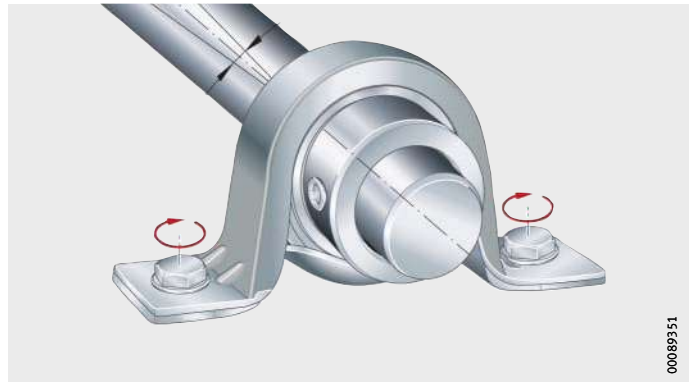
Figure 12 Screw mounting the housing finger tight
