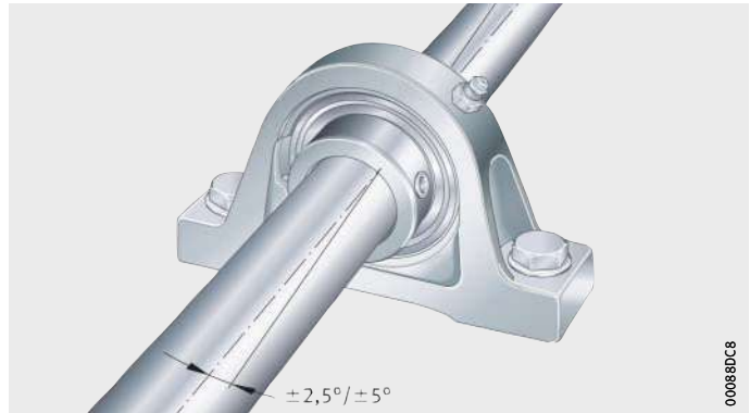
Figure 5 Compensation of static shaft misalignment
