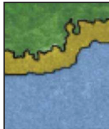
■ Sealing ■ Adhesion layer ■ Aluminium surface
