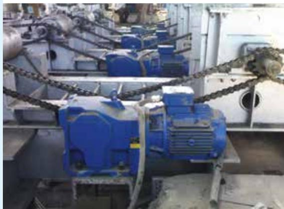
Bevel geared motor for cooling bed - chain transfer table
