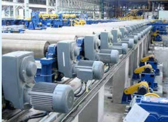
Parallel shaft geared motors for roller tables
