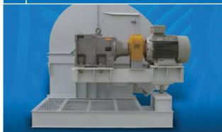
Screw Feeders are used to move bulk materials from silos, hoppers or bins. Screw Conveyors incorporate a screw rotating in a housing to transport the material. The bulk material flows forward with each revolution of the screw and is can be metered through the shroud for accuracy.
