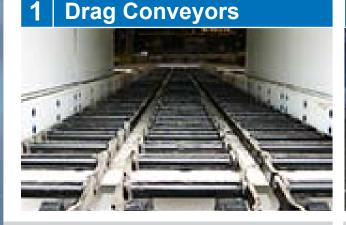
Drag conveyors can be used to meter or transfer bulk materials from one process to another. The design and characteristics of the drag conveyor enables it to fit almost any plant layout and is ideally suited to handle dry, free-flowing materials. A primary benefit of the drag conveyor include little product degradation during conveying and require less horsepower than other types of conveyors.
