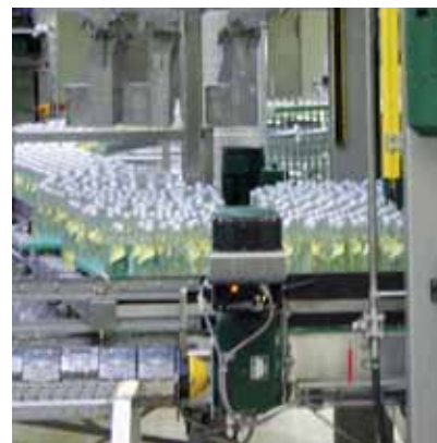
Left: NORD drive units are mounted on both sides of the conveyor belt.
