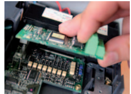
Connector system for time-saving installation
