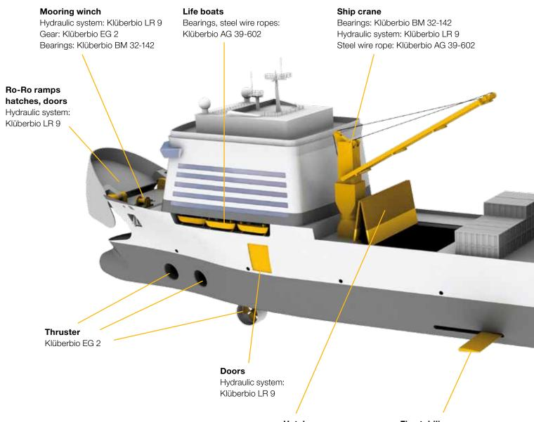
This illustration shows the various applications of our marine lubricants. To show as many applications as possible in one illustration, we included components of the following ship types in this synthetic ship: Ferry, cruise ship, cargo ship, wind turbine installation vessel, anchor handling tug supply vessel.
