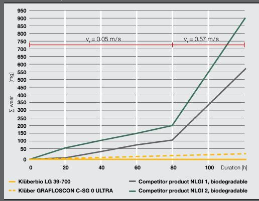
Klüberbio LG 39-700 shows lower wear rates than other open gear lubricants.
