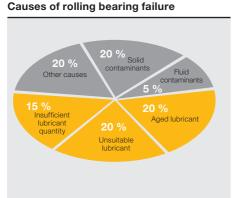
55 % of rolling bearing failures could be prevented through the use of Klübermatic lubricating systems!
