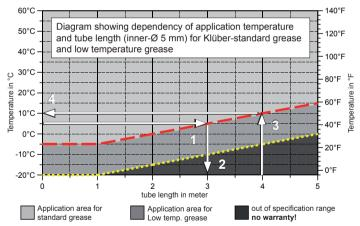
The dashed standard grease- and dotted low temperature-lines show the maximum values allowed.
