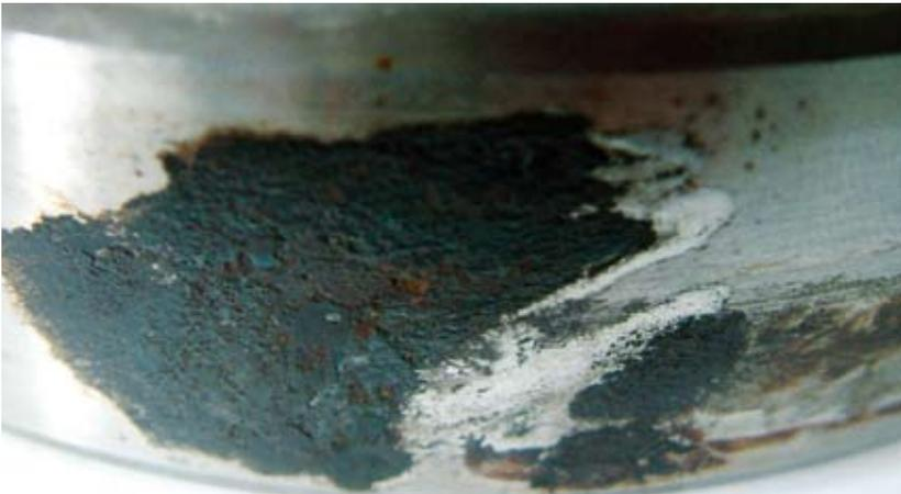
Fretting corrosion on the outer ring
