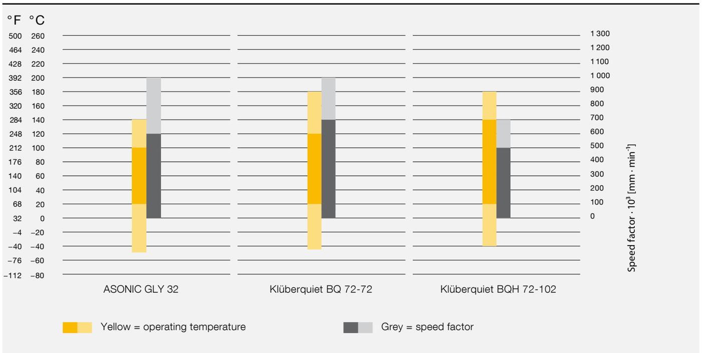
The operating temperature range and the maximum speed factor  $n \cdot d_m$  can be read from the diagram. The darker areas are the target if lifetime lubrication is required.
