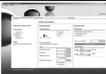
Which electromechanical linear drive best meets your needs? Enter the data for your application, such as position values, effective loads and mounting position, and the software suggests a number of solutions.
