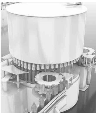
Machine parts and components in the splash zone come into direct contact with food. The food cannot be returned to the product flow from this zone. However, the splash zone should still be planned and designed according to the same criteria as the food zone – even if the product cannot be returned to the food process. The technical implementation can be less stringent, provided this does not have an unfavourable effect on the quality of the manufacturing process.
