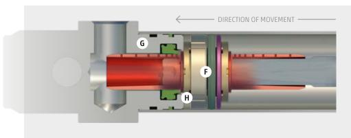
The movement stops when the end stroke position is reached and the piston **(F)** touches the end block **(G)**. The presence of a damper (H) absorbs any residual kinetic energy and minimises the impact so that there is no vibration or noise.
