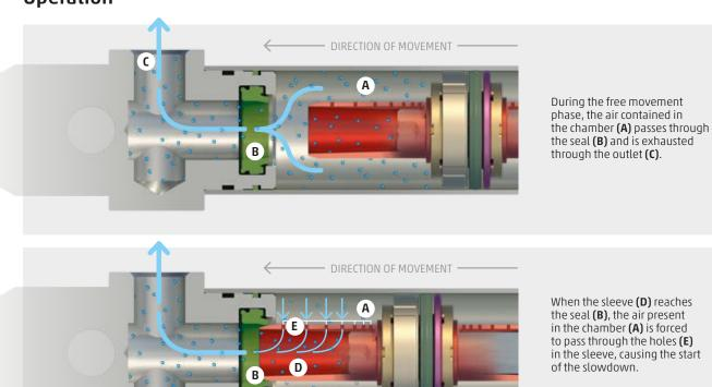
When the sleeve (D) reaches the seal (B), the air present in the chamber (A) is forced to pass through the holes (E) in the sleeve, causing the start of the slowdown.
