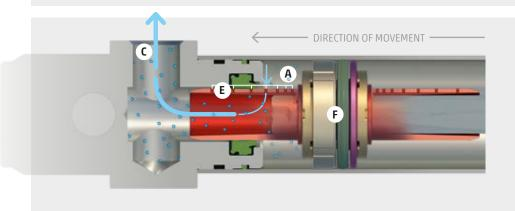
As the piston (F) moves, the holes (E) close off one by one causing a consequential decrease in the air flow from the chamber (A) towards the outlet **(C)**, generating a progressive and smooth deceleration.
